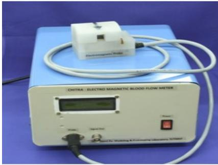
The device is a portable, battery-operated, fluid flow meter for measuring flow of blood or conductive fluids in an extracorporeal circuit during bypass surgeries. It has very high sensitivity, zero warm-up time, minimum signal drift, lower heat dissipation and minimal power losses. The blood flow meter consists of a flow tube sensor, which is attached to the extracorporeal circuit. The device displays the flow in its display unit as litres/min.
