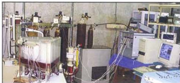
Experimental set up for in vitro evaluation of membrane oxygenator
