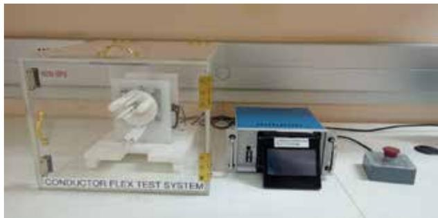
Figure 48. Conductor flex testing
