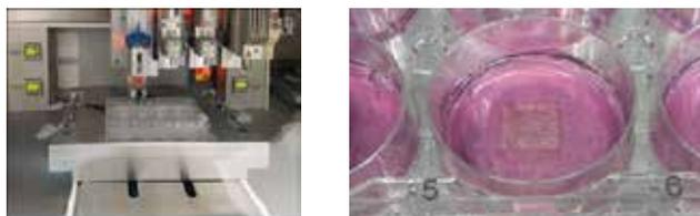
Figure 10. 3D bioprinting of liver construct using RegenHU 3D Discovery bioprinter using bioink characterized for hepatocyte printing (10A) and 3D bioprinted liver construct (10B)
