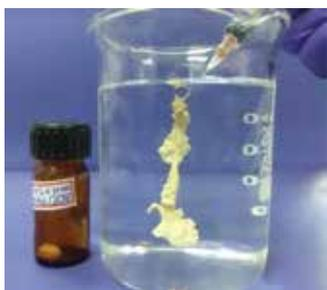
Figure 50. Precipitation behaviour of radiopaque liquid embolic agent in saline
