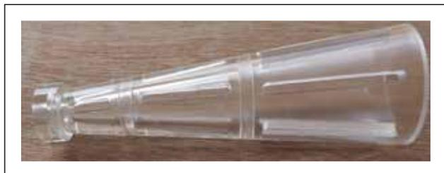
Crimping former fixture to crimp aortic stent graft prototype
