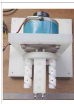
Conductor flex test setup fixture
