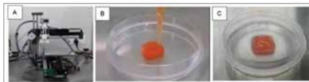
Figure 4. (A) Customised 3D Bioprinter, (B) liver construct printed using in house developed bioink with rat hepatocytes and (C) the construct after 14 days of in vitro culture
