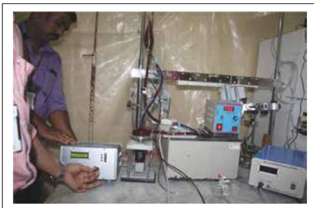
Figure 18. In vitro evaluation of centrifugal blood pump using blood
