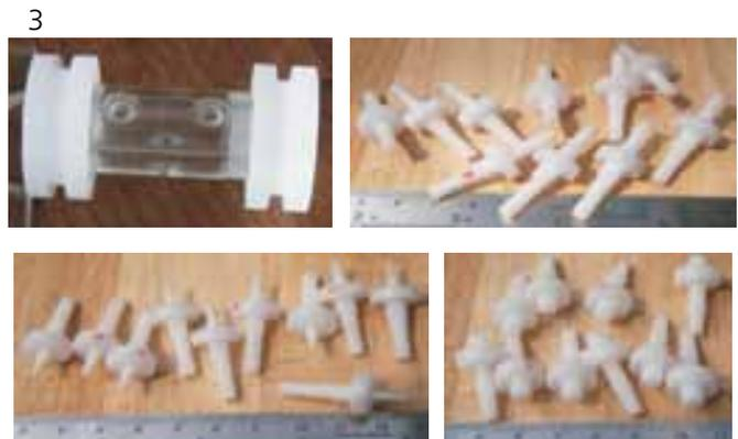
Completed the machining of Bioreactor components and connectors to Tissue culture lab
