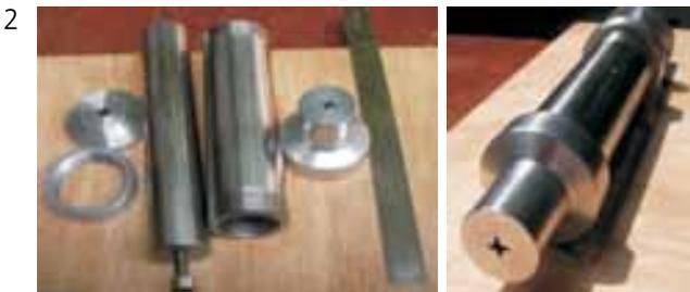
Completed the designing and machining of ceramic slurry extruder setup for Bioceramic Lab
