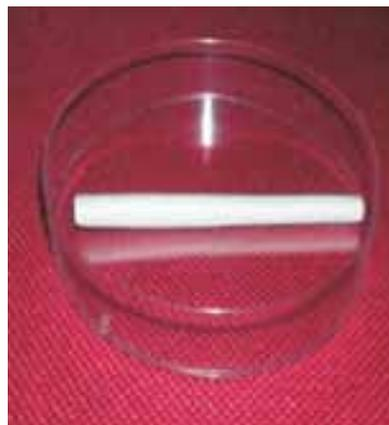
Small diameter vascular graft with optimum porosity developed in DPL
